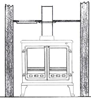
Typical Rear Flue Installation with clean out door
