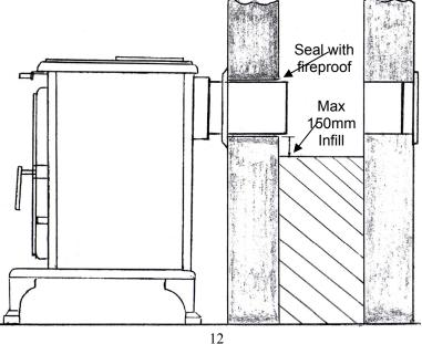
An existing fireplace opening can be bricked up or sealed with a register plate, 1.5mm steel sheet or concrete. A short length of flue pipe no smaller in diameter then the stove flue outlet or the manufacturer's stated flue size may then be used to connect the stove to the chimney. This flue pipe should be of cast iron, 316 grade stainless steel or vitreous enamelled, nominal thickness 1.2mm. Ensure that the pipe end is no closer than 76mm to the side or rear chimney walls.
